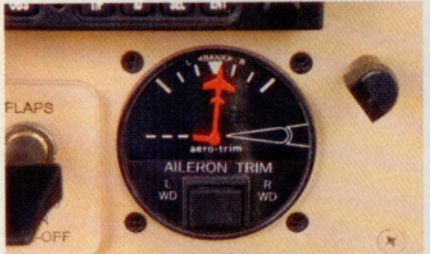
The AeroTrim electric trim gauge manages any imbalance in aileron pressure.
